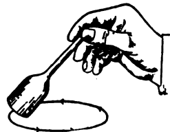
FIG. 17.—To mix the acid and milk whirl the bottle in a circle until the contents are of a uniform brown color.
